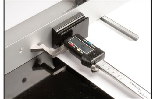
With the digital height gauge placed horizontally on your router table top and up against the fence, slide the foot until it touches the router table fence surface. Press the zero button and the readout should read all zero's.
