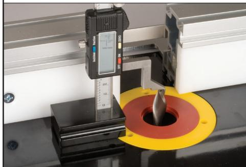
Set the gauge to your desired height and lock into position with the locking knob. Place the digital height gauge next to the router bit with the foot directly above the bit. Raise the bit until it just touches the base of the foot.
