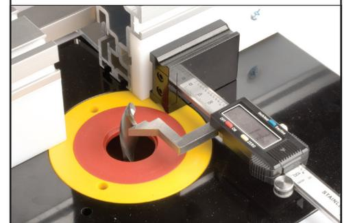
Set the gauge to your desired router bit distance from your fence and lock into position with the locking knob. Place the gauge horizontally on your router table top and up against the fence. Adjust the fence so the foot just touches the desired point on your router bit.
