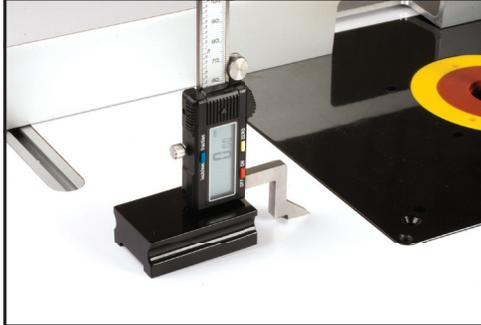
With the digital height gauge placed on your router table top, slide the foot down until it touches the table top surface. Press the zero button and the readout should read all zero's.
