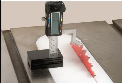
Set the gauge to your desired height and lock into position with the locking knob. Place the digital height gauge next to the saw blade with the foot directly above the blade. Raise the blade until it just touches the base of the foot.
